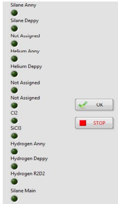
Figure 9 The LabVIEW code for individual control of solenoid valves for gas flow
