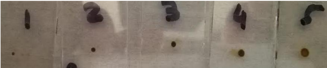
Figure 21 Effect of increasing the distance between the nozzle and the substrate on the deposition profile. The distance is increasing from 0.7cm to 3.2cm, going from 1 to 5.
