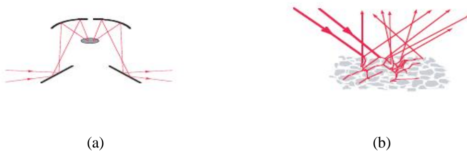
Figure 19 (a) Schematic of DRIFTS accessory, (b) Schematic of diffuse reflectance from a powder [27]
