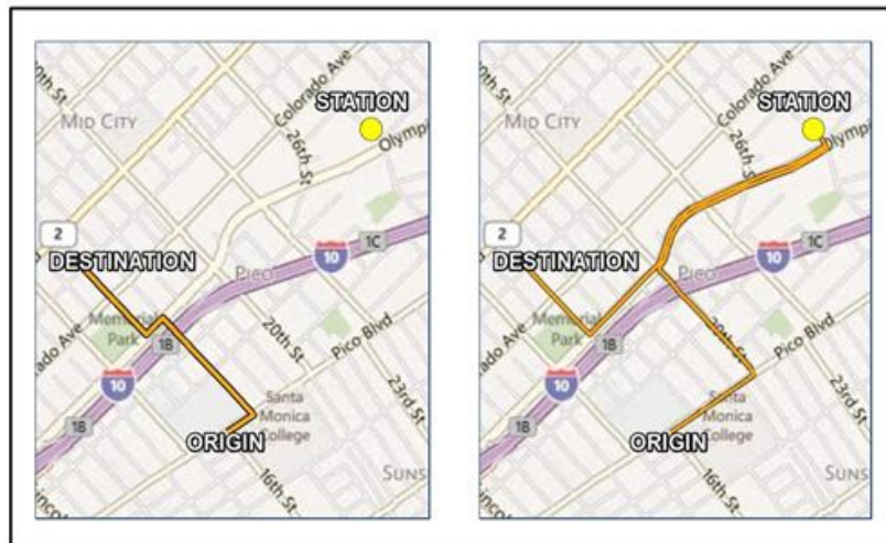
Figure 2.2. Comparison of least travel-time direct path and refueling path, which forms the basis for deviation calculations.
