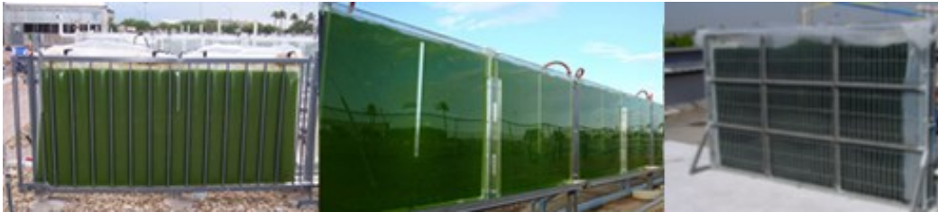
Figure 2.5: Left: photo of Pseudocolumn Reactor at AzCATI Facility. Center: photo of research scale flat-panel reactors at AzCATI. Right: Photo modified from Acién Fernández et al. (2013) of design patented by Tredici and Rodolfi to minimize variation in light-path length.
