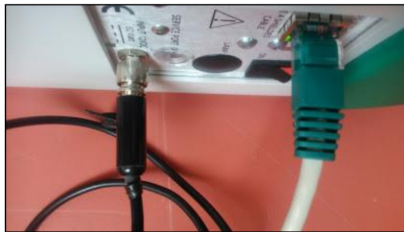
Figure B1. Power supply to port connection
