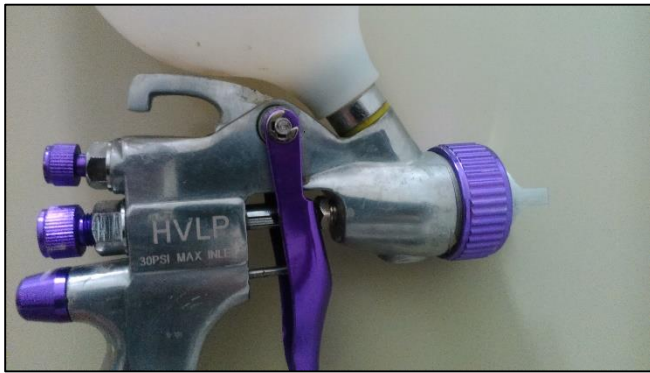
Figure 8. Spray Gun (a) Without Laser Pointer
