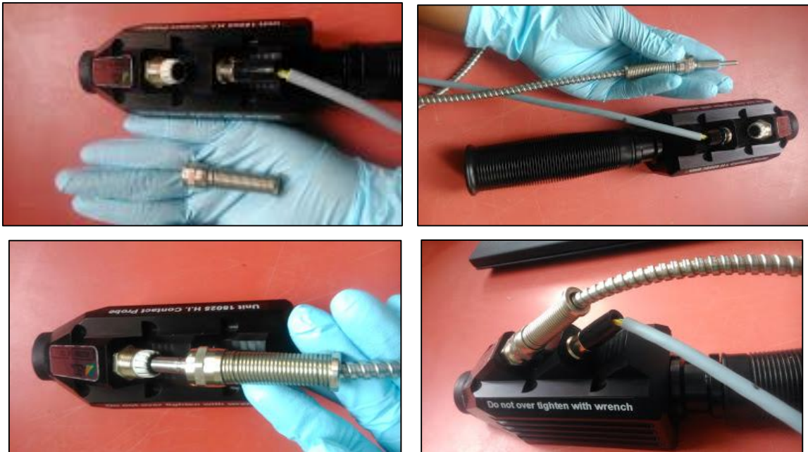
Figure B3. Step-by-step process of inserting optic fiber to the contact probe
