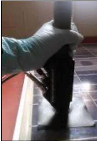
Figure B9. Reflectance measurement on module
