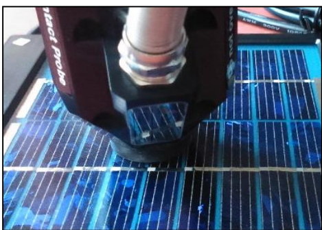
Figure 14. Reflectance Measurements on (a) Poly-Si
