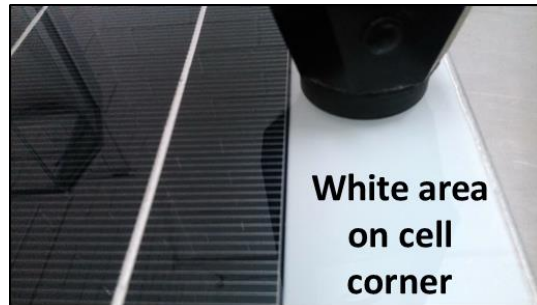
Figure 25. Contact Probe on White Area for Reflectance Measurements (see Figure 16 for the full size picture of the 1-cell coupon)
