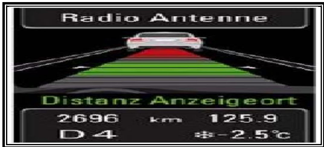
Figure 6.2: LDWS Info on the Instrument Panel of Audi A4
