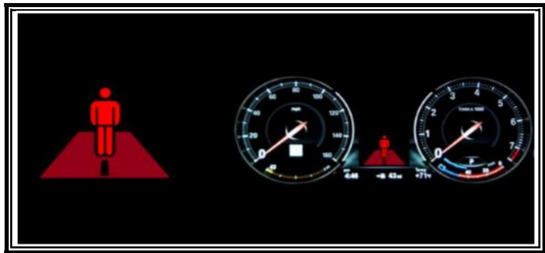
Figure 6.4: Pedestrian Detection Warning in the Instrument Cluster
