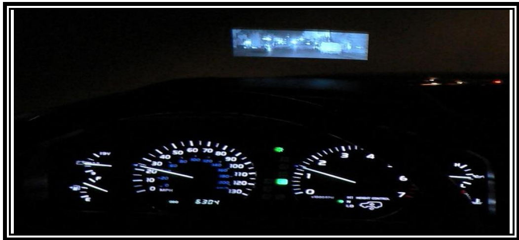
Figure 6.10: NVS HUD Introduced on Toyota Lexus LS600
