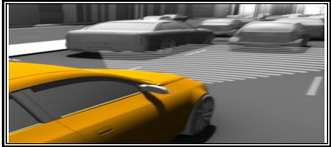
Figure 6.7: ACC Sensors Monitoring the Vehicles Ahead
