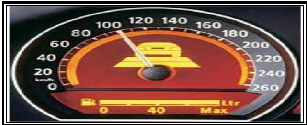
Figure 6.8: ACC Lights When Approaching a Slower Car
