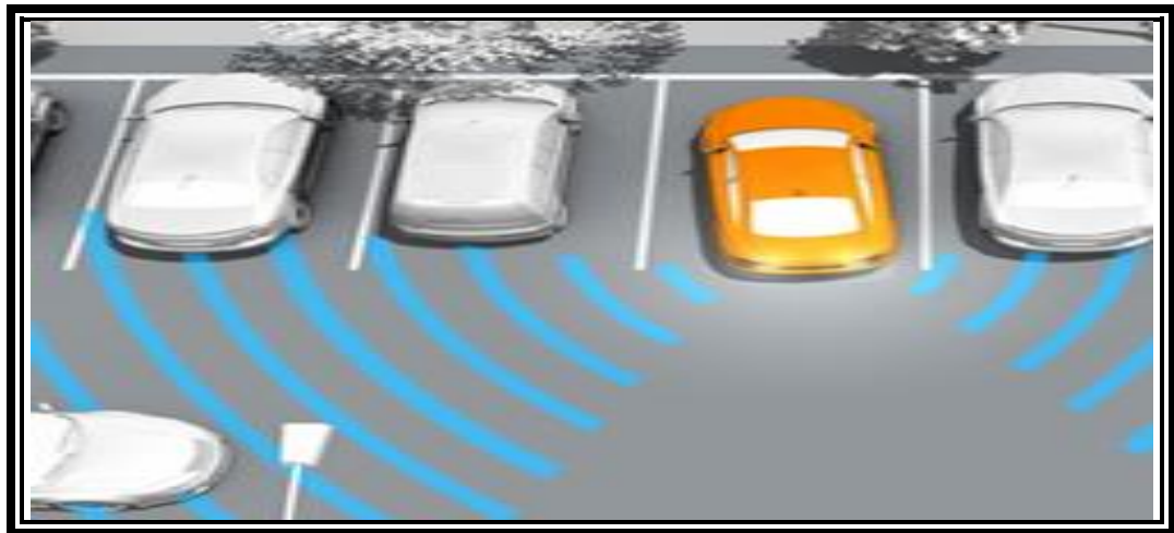
Figure 6.6: RCTA Sensing While Reversing
