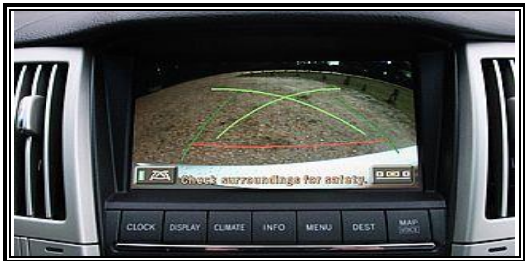
Figure 6.9: Lexus Backup Camera Showing the Parallel Park Setup
