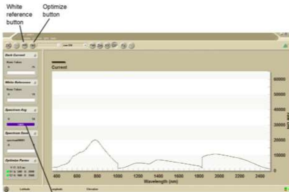
The software starts collecting spectra immediately. The Spectrum Avg progress bar shows the spectra collection.
