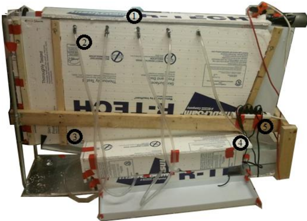
Figure 18. Completed Unit 2 with insulation over the pumps and a short brine exit box beside the pumps.
