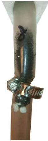
Figure 14. Clamps and reticulated foam to address Challenge 5.
