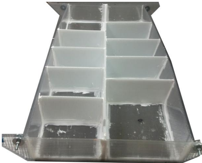
Figure 16. Second basin built with segments to reduce mixing.
