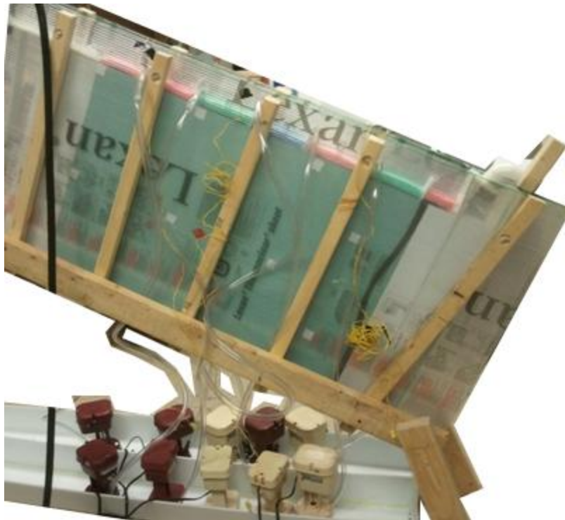
Figure 13. Vertical wooden side braces to address Challenge 4.
