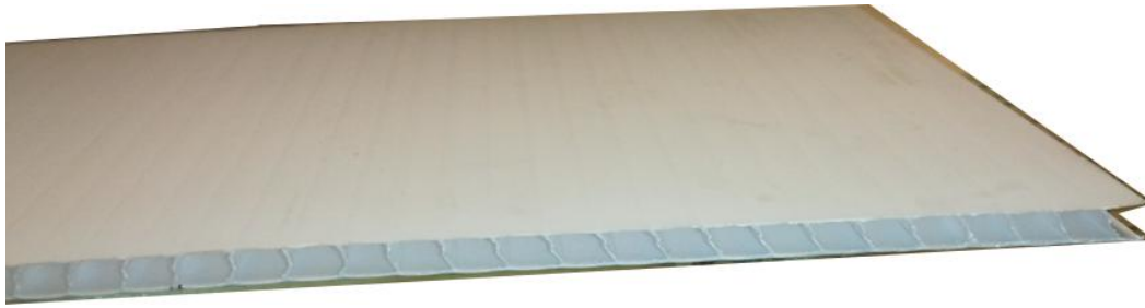
Figure 6. Twin-wall extruded polypropylene.
