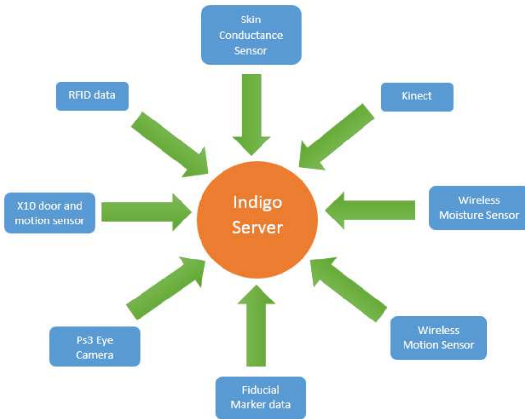
Figure 21. Information flow from different components to the central server
