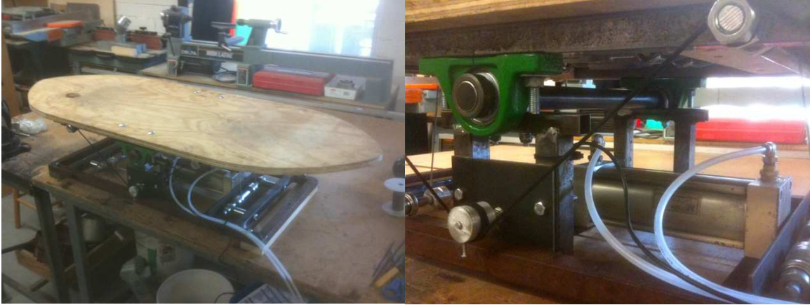
Figure 6. Physical Function pneumatically actuated balance interface (left) and detail showing pneumatic and position sensor components (right).
