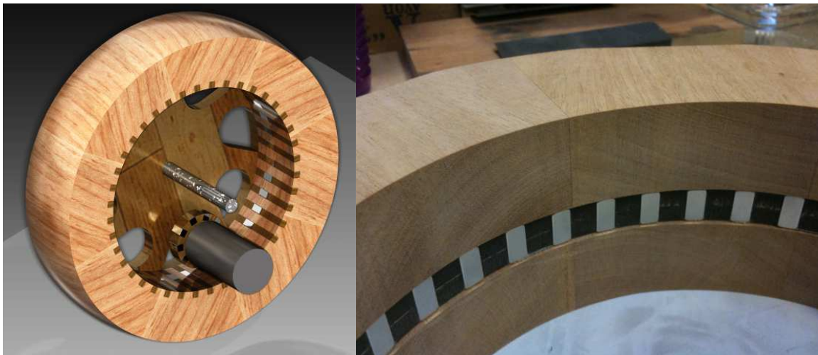
Figure 21. Vox Curio flywheel 3D model (left) and detail of actual flywheel in production, showing array of embedded magnets.
