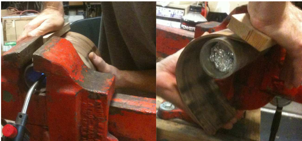
Figure 13. Bending walnut panel over heated aluminum cylinder for body of Vox Curio instrument.
