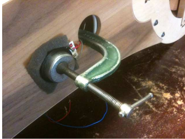
Figure 24. Testing a vibrotactile actuator on the acoustic body of the Vox Curio instrument.
