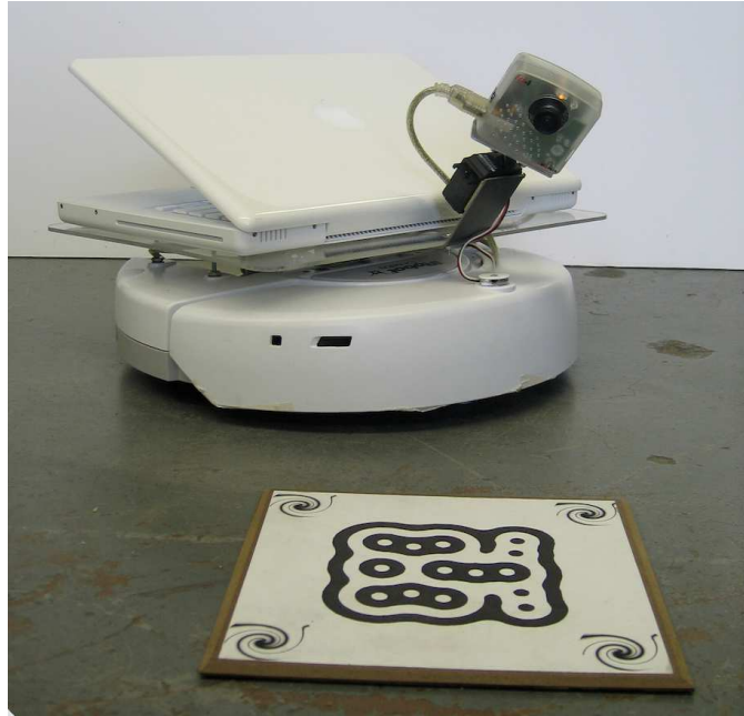
Figure 3. An ALERT robot reacting to a tangible fiducial programming instruction.
