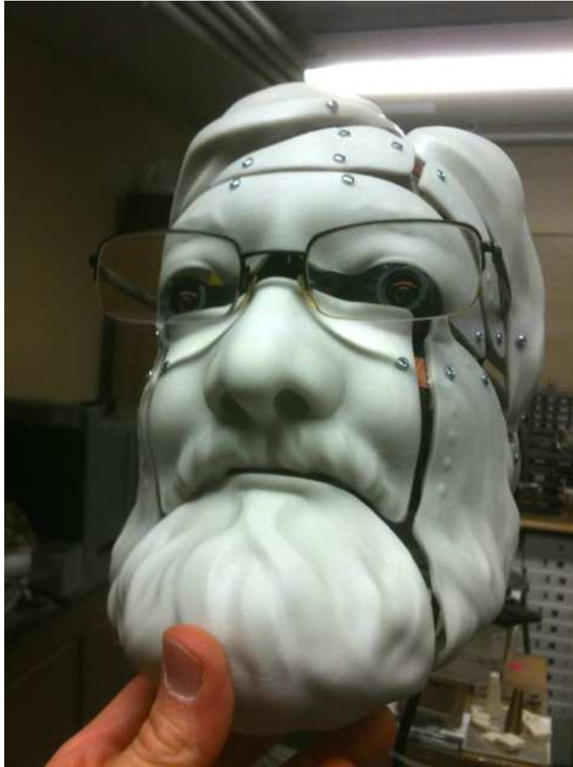
Figure 9. Animatronic head of PeteBot featuring embedded audio/video sensors and servo motor actuators.
