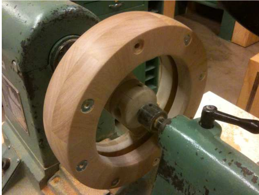
Figure 16. Re-fabricated mahogany flywheel mounted in wood lathe.
