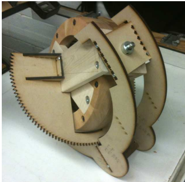
Figure 22. Assembled 'control moment gyroscope' head of Vox Curio instrument.
