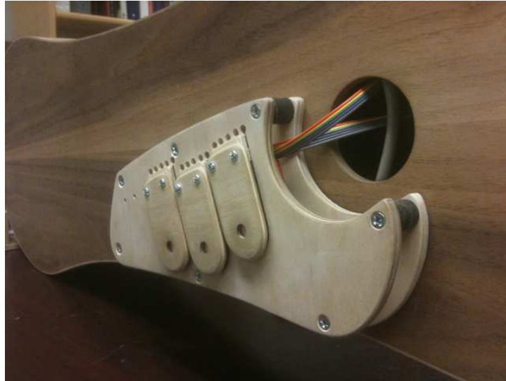
Figure 25. Vox Curio 'valve' pressure sensor/actuator assembly attached to instrument body.
