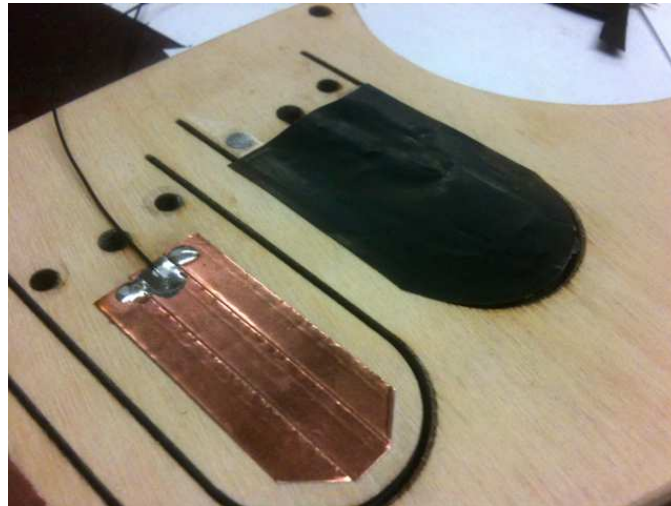
Figure 26. Vox Curio 'valve' pressure sensors under construction. Copper tape and Velostat material are visible.
