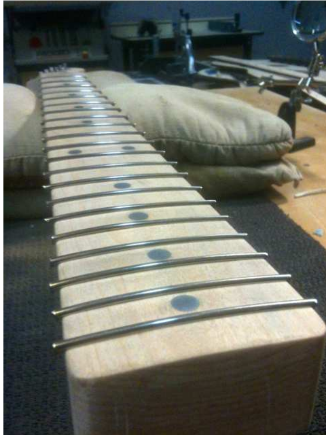
Figure 30. Guitar neck in production, showing end grain orientation.
