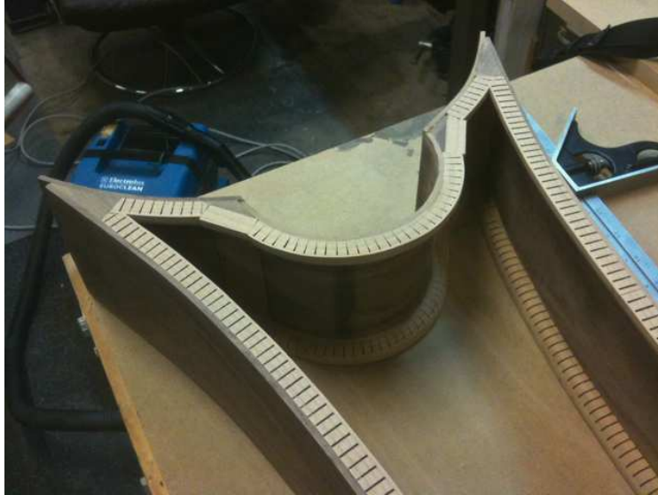
Figure 17. Kerfing installed on the interior edges of Vox Curio in preparation for the attachment of the top and back panels.
