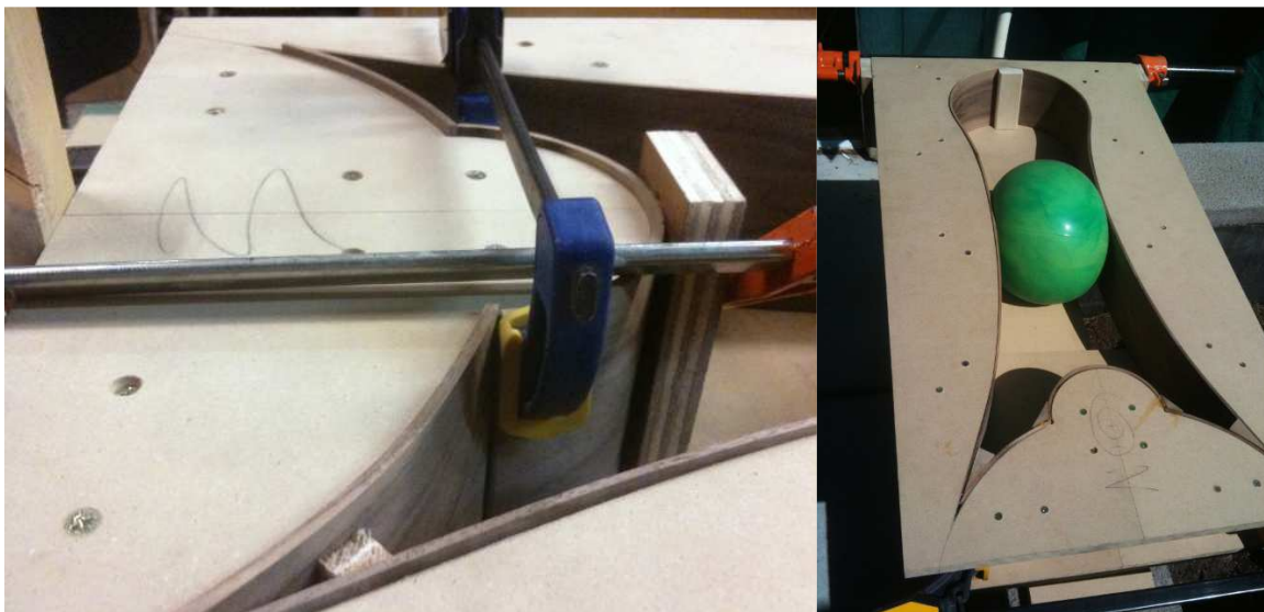
Figure 14. Bent wood pieces clamped in structurally defining form with bar clamps (left) and with rubber ball (right).
