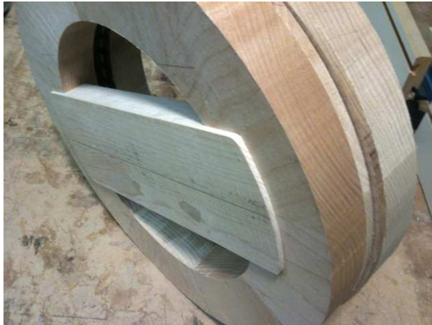
Figure 15. Original, unfinished, flywheel that eventually broke. Maple crossbeam can be seen diagonally spanning the diameter of the flywheel.
