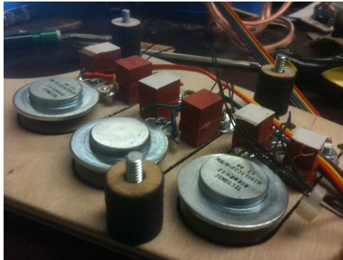
Figure 27. Detail of vibrotactile actuators on Vox Curio instrument 'valves'.
