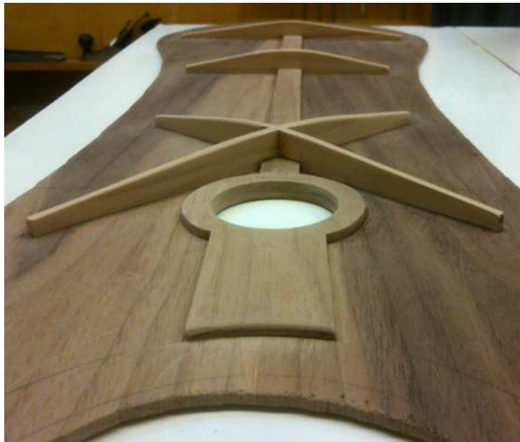
Figure 18. Structural bracing installed on underside of top panel of Vox Curio instrument.
