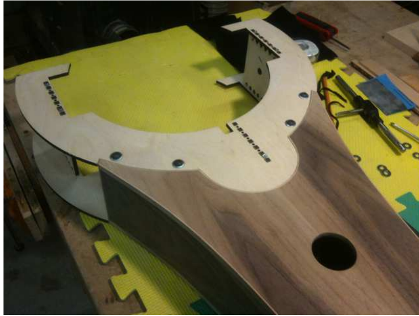
Figure 20. Integration of hand built and laser cut subassemblies of Vox Curio instrument.
