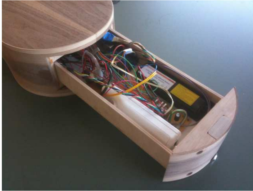
Figure 23. Electronics drawer partially inserted into Vox Curio instrument body.
