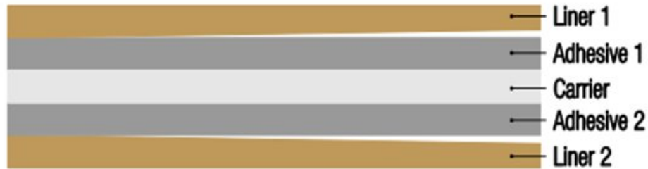
Figure 14. Spacer construction with material specification [69]
