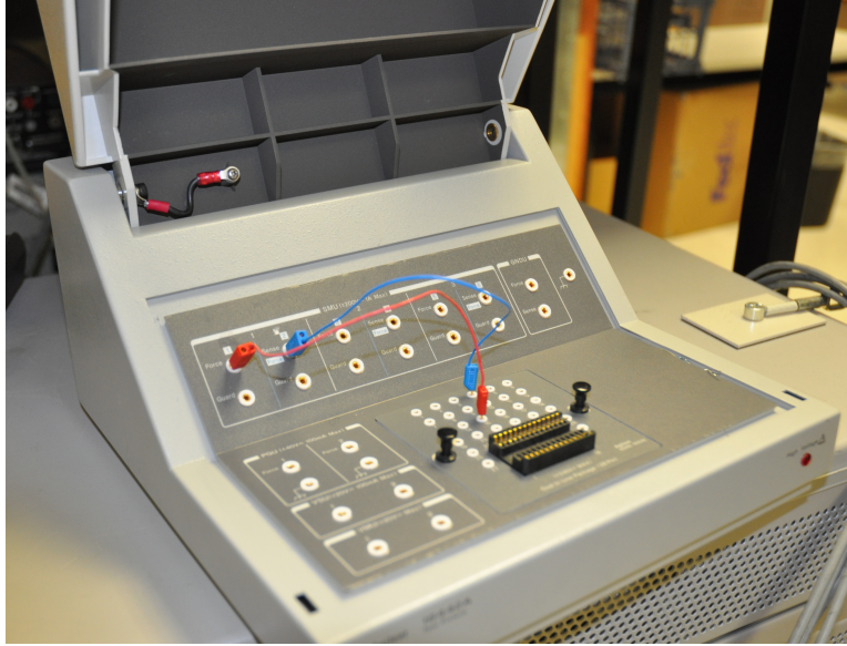
Figure 4.2: Test fixture used for performing automated electrical measurements.
