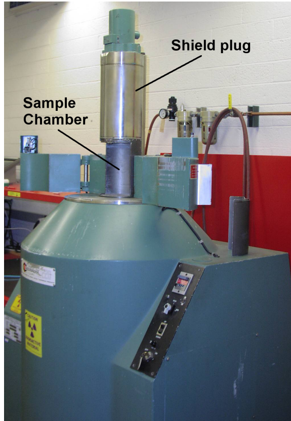
Figure 4.3: The Gammacell 220 used for \gamma -ray exposure. Photo provided by Dr. Keith Holbert.
