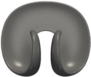
Figure 42 - Fluid interface halfway through the test case, when t = 1.5 , after the sphere is initially deformed using the operator-split rotational advection scheme for transportation.
