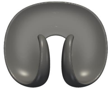
Figure 42 - Fluid interface halfway through the test case, when t = 1.5 , after the sphere is initially deformed using the operator-split rotational advection scheme for transportation.
