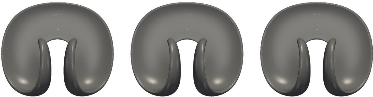
Figure 37 - Fluid interface halfway through the test case, when t = 1.5 , after the sphere is initially deformed using the operator-split non-rotational advection scheme for transportation.
