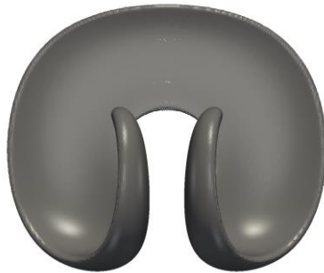
Figure 42 - Fluid interface halfway through the test case, when t = 1.5 , after the sphere is initially deformed using the operator-split rotational advection scheme for transportation.
