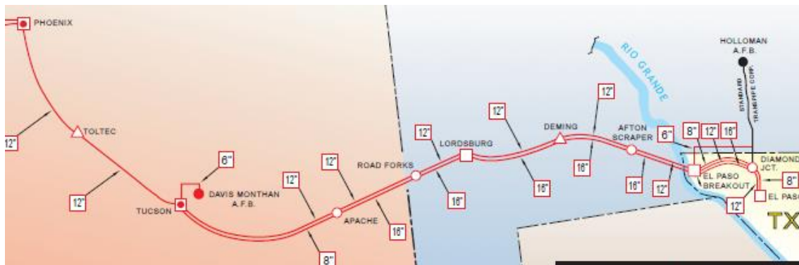
Figure 26. Phoenix Fuel Supply - East Line
