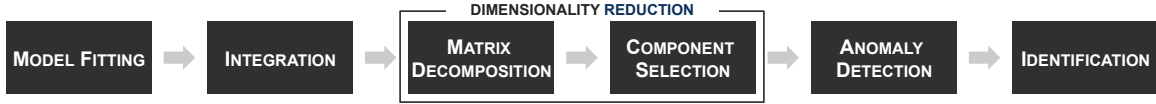
Figure 4.1: Extending SPG Framework for Dynamic Graphs. The input into the SPG framework is now a set of adjacency matrices A , where each matrix A_t represents the dynamic graph at time interval t , G_t . A new algorithmic step is added following the model fitting step to allow for temporal integration. The rest of the framework remains the same. The output of the algorithmic steps, as in the static case, is the vertices identified as part of the anomalous subgraph.
