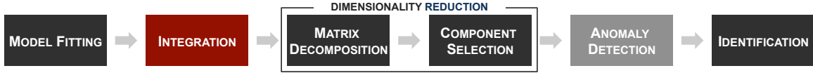
Figure 6.3: SPG Block Diagram - Author Detection Relevant Blocks. To identify key author subgraphs, we applied the model fitting/residual computation step, temporal integration step, dimensionality reduction step, and identification step to a dynamic, temporally evolving collaboration network. Since the focus of the work presented is the temporal integration, that algorithmic block is further highlighted.
