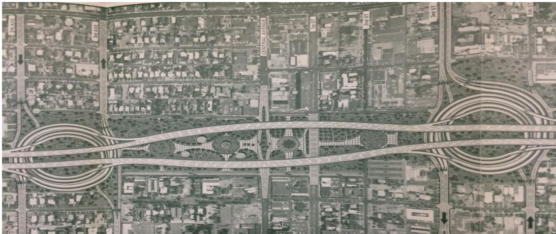
Figure 9. The Papago Free Elevated Concept Design. The image shows the elevated concept design of the Inner Loop with the helicoids. 201
