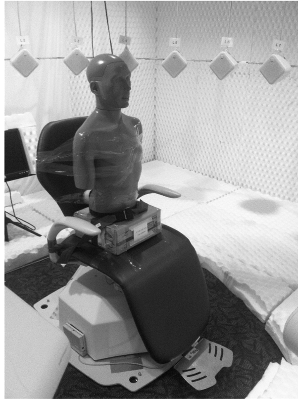
Figure 6.5. The test setup of KEMAR on a rotating chair in the middle of the test room.
