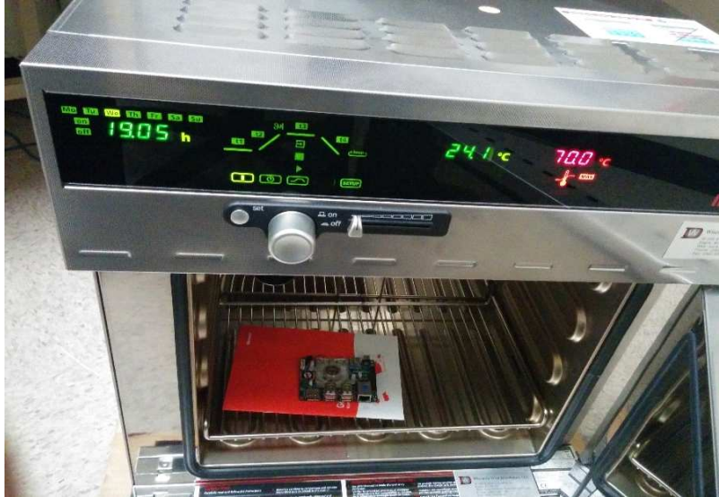
Figure 4.1: Temperature furnace used to model leakage power
