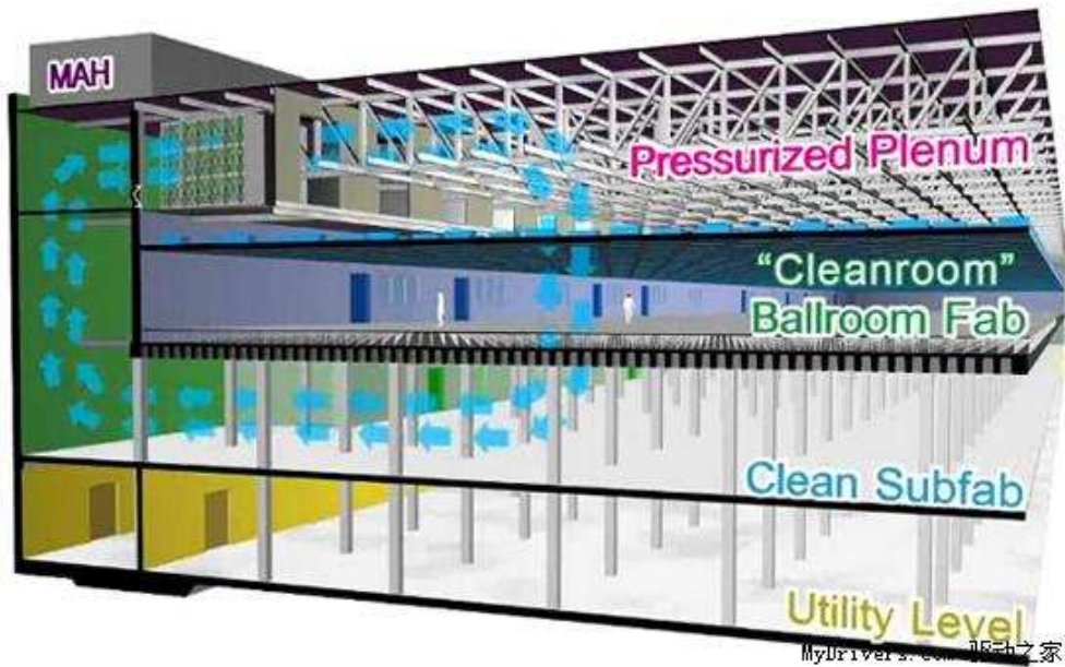
Figure 12. Cross-section of a Wafer Manufacturing Fab. Reprinted from Intel/Micron 25nm process fab day tour by Shu, 2010
