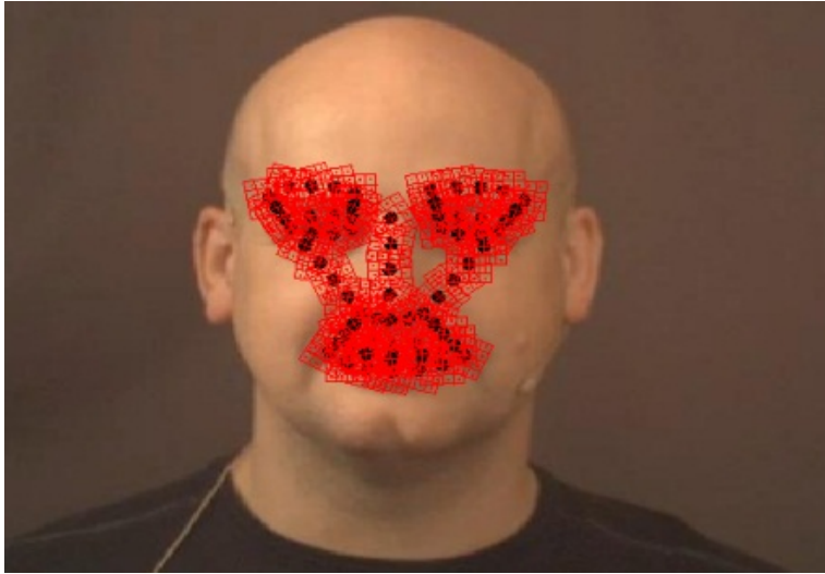
Figure 3.5: Plot of SIFT [39] features extracted from 71 interpolated facial fiducial points
