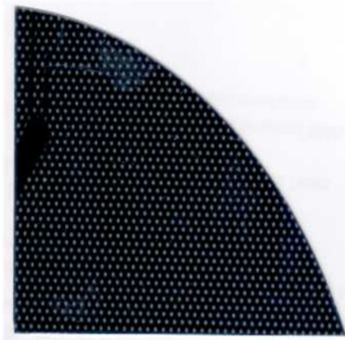
Figure 3.7. MOS capacitors fabricated on the surface of the wafer with circular Aluminum gates deposited with PVD and through a shadow mask.
