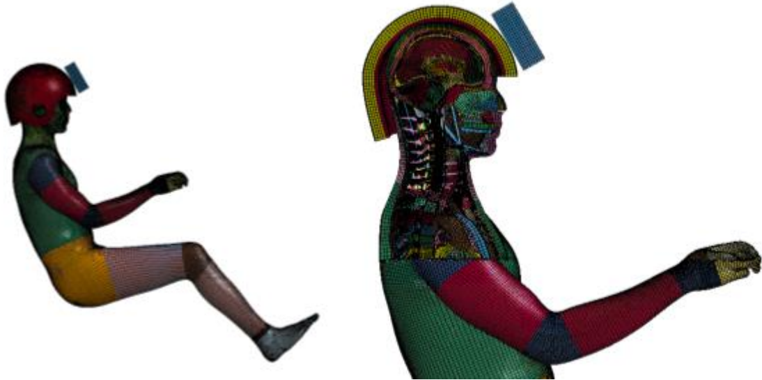
Figure 18 GHBMC Model Integration: (a) full GHBMC model integrated with the football helmet model and impactor. (b) Cross section of the GHBMC to note anatomical detail.
