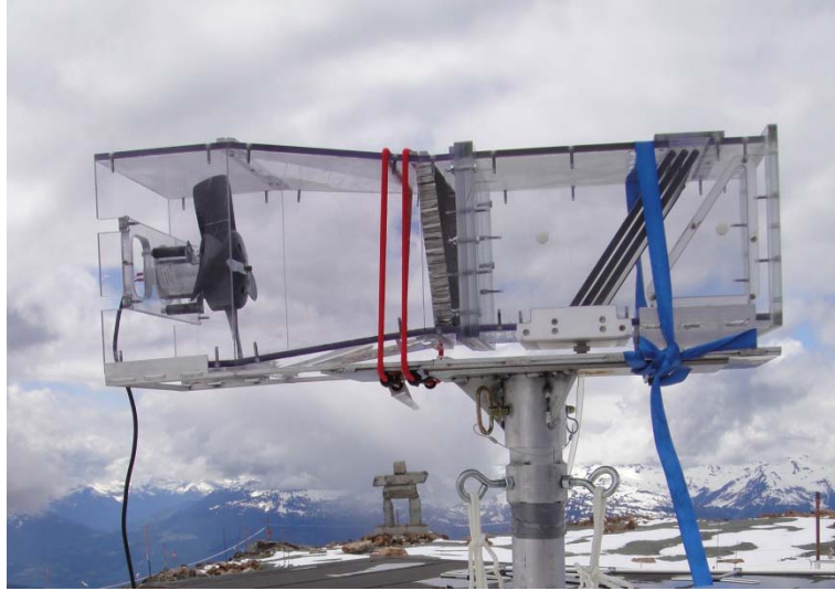
Fig. 1.2 A single stage Caltech Active Strand Cloud water Collector being used on top of Whistler mountain, Canada.
