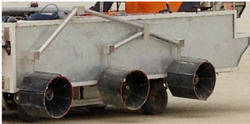
Photograph 14. The Rocker-bogie Suspension System. Photo by author.
