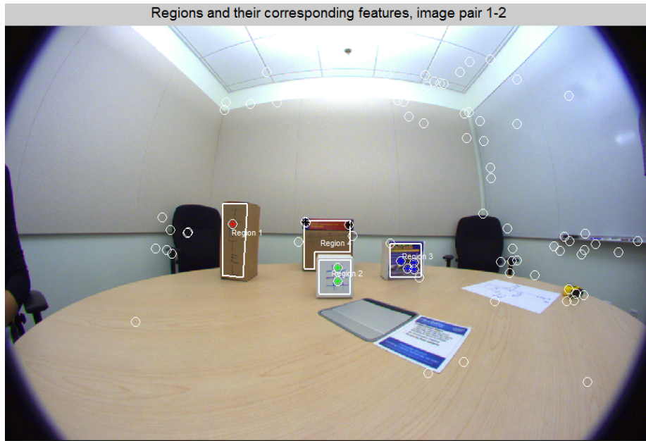
Figure 6.6: Regions of known depth enclosed by white rectangles and their corresponding feature points.
