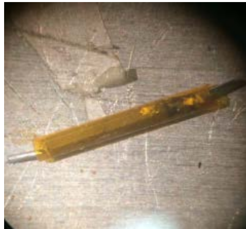
Figure 23 Device Fit Through Polyamide Tube
