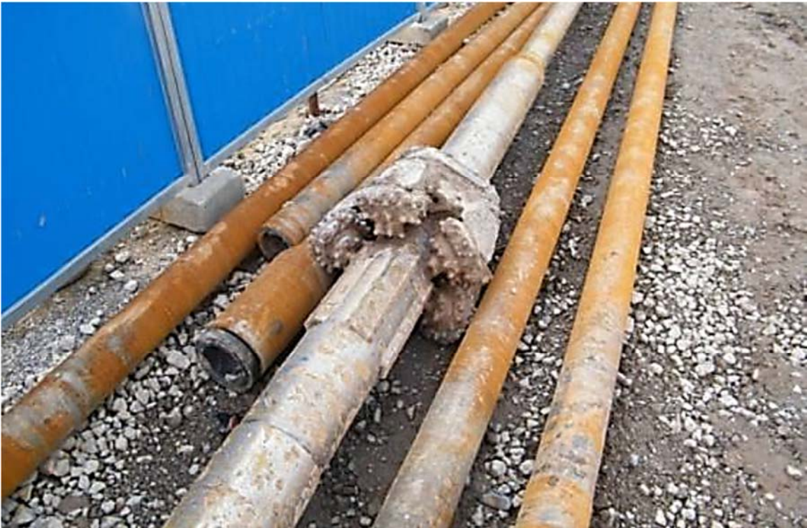
Figure 5.37: Stuck Reamer (Li et al, 2013)
