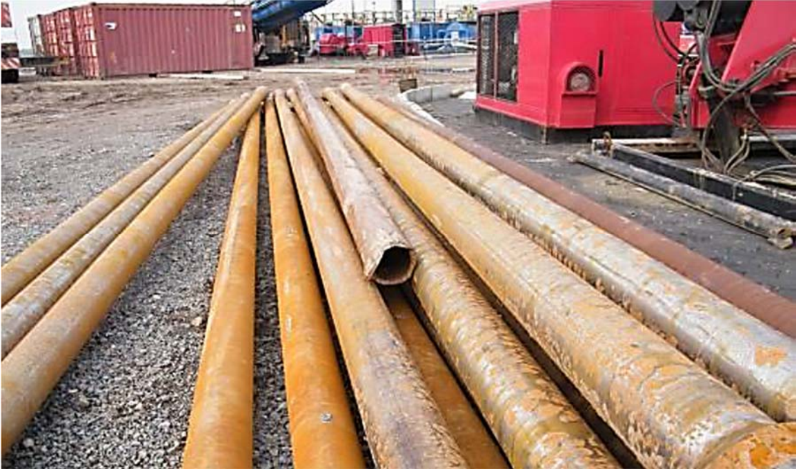
Figure 5.36: Broken Drill Pipe (Li et al, 2013)
