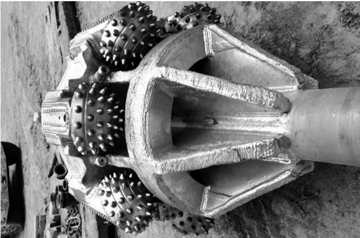
Figure 6.23: Refurbished Galvanized Mill-Tooth Reamer (Laney, 2014)
