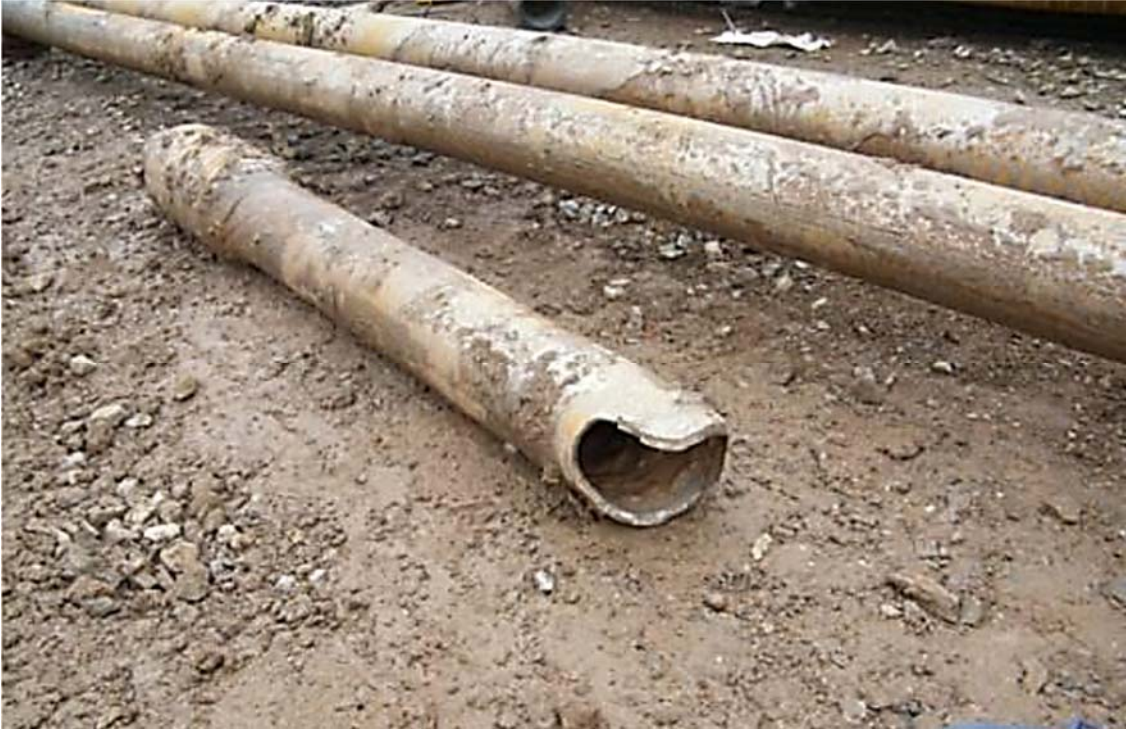
Figure 5.38: Fractured Drill Pipe (Li et al, 2013)
