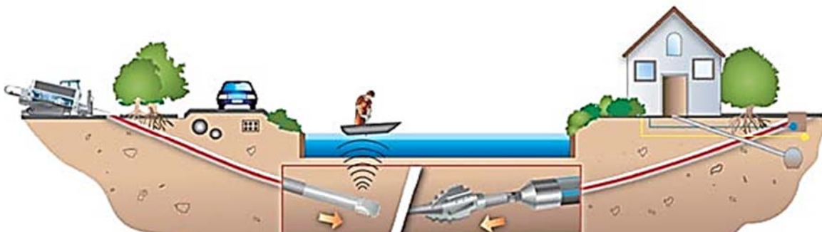
Figure 2.3: HDD Schematic (Tracto-Technik GmbH & Co. KG)
