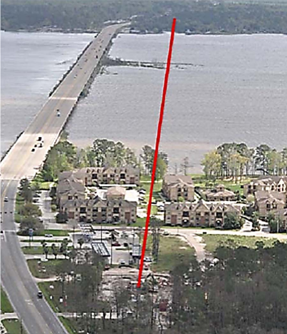
Figure 5.41: Alignment of Drill Path Across River (Laney 2013)
