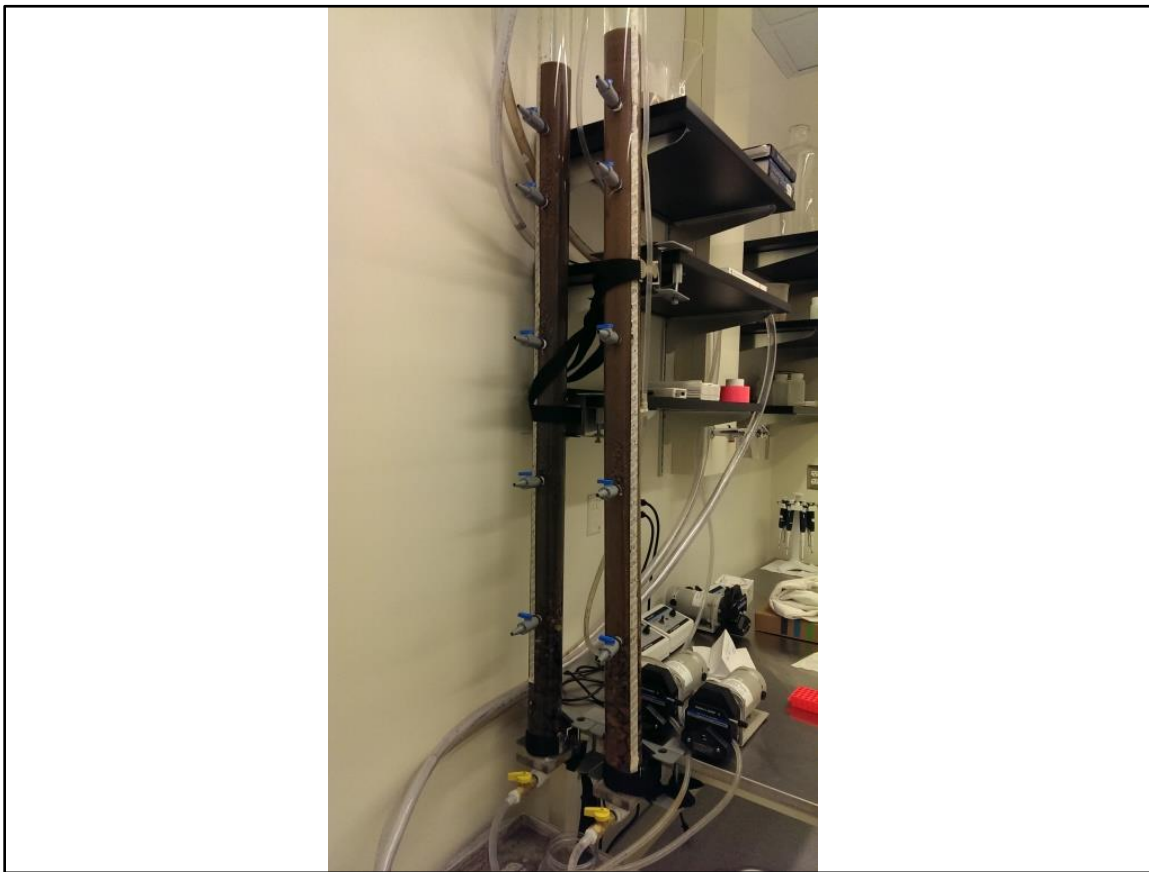
Figure 3.12 Column A (left) and B (right) Packed with Central AZ Recharge Media
