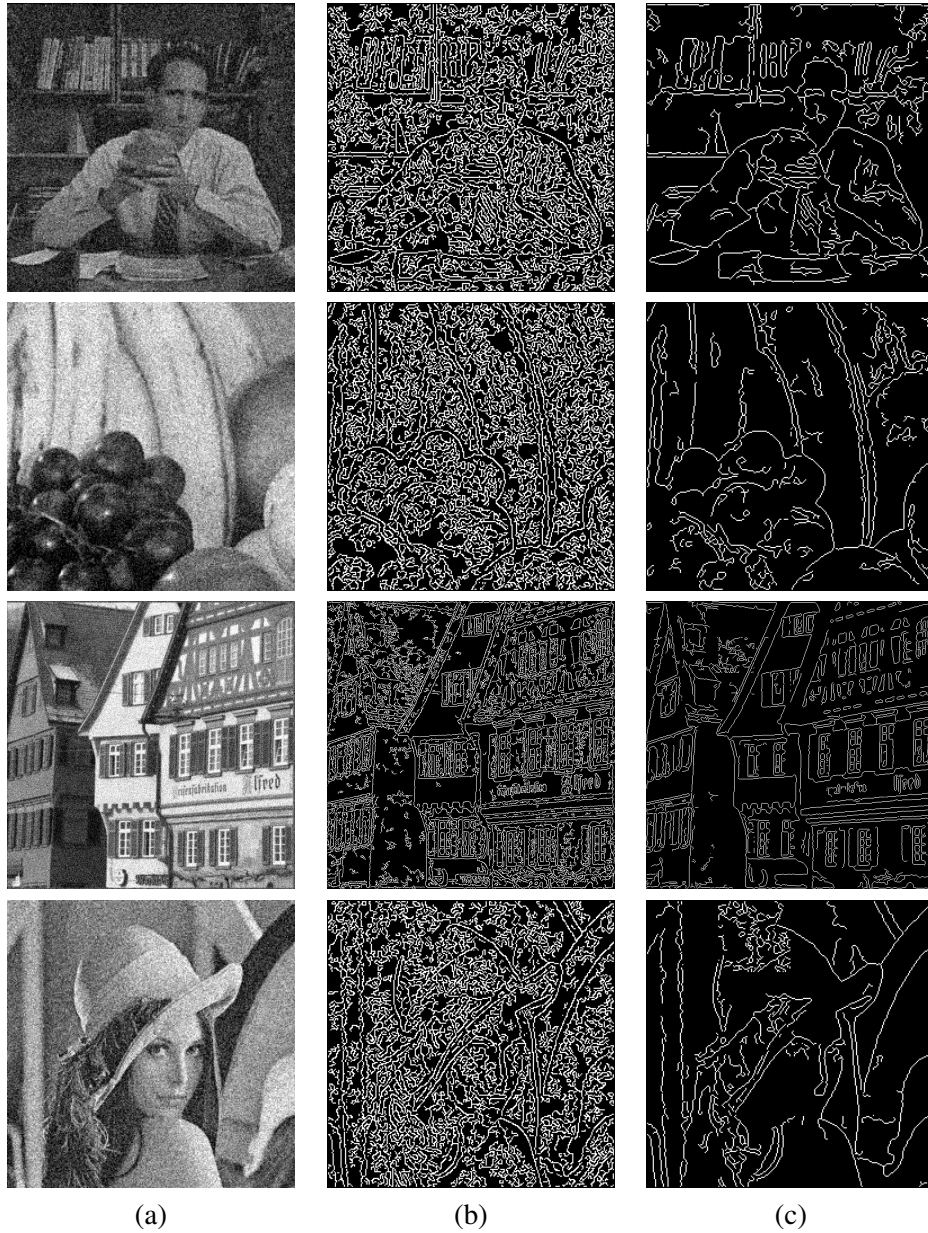
Figure 3.18: Comparison of the Edge Maps of Noisy Images by Using the Original Canny Edge Detector And the Proposed Method: (a) Images with Gaussian White Noise ( \sigma_n = 0.01 ); Edge-Maps of (b) the Original Canny Edge Detector, And (c) the Proposed Algorithm with A Non-Overlapping Block Size of 64 \times 64 , Using A 9 \times 9 Gradient Mask.
