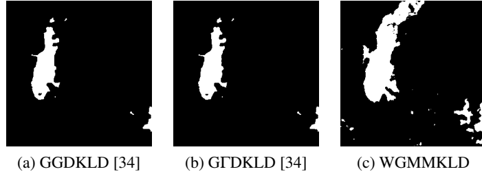
Figure 5.20: Change Detection Results from Different Wavelet-Domain Algorithms on the Bangladesh SAR Image Dataset With A Window Size Of 5 \times 5 And Scale=3.
