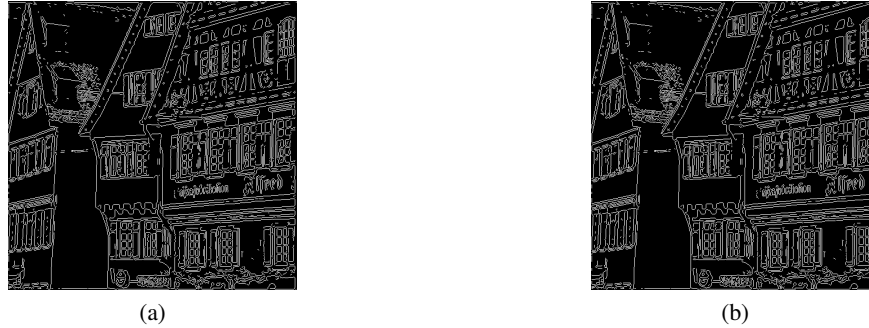
Figure 3.26: Comparison between the Fixed-Point Matlab Software Simulation Result And FPGA Hardware Simulation Result For Detecting Edges of the 512 \times 512 Houses Image Using A Block Size of 64 \times 64 And A 3 \times 3 Gradient Mask: (a) Edge Map Generated by the Fixed-Point MATLAB Implementation; (b) Edge Map Generated by the FPGA Implementation.
