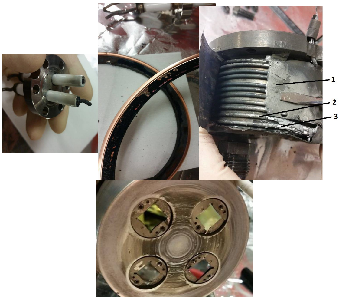
Figure 13: Examples of corroded UHV chamber components. Left: remnants of Cu power-feedthrough after ~6 months of use. Center: Corroded UHV flange Cu gaskets after <24 hours at room temperature in SE chamber. Right: stainless steel substrate heater; 1) corroded stainless steel sheet metal, 2) inconel sheath of heating element, 3) exposed MgO powder insulation as a result of corrosion damage to inconel sheath. Bottom: Grooved tracks in rotating substrate heater, indicating that metal is being removed by corrosion.
