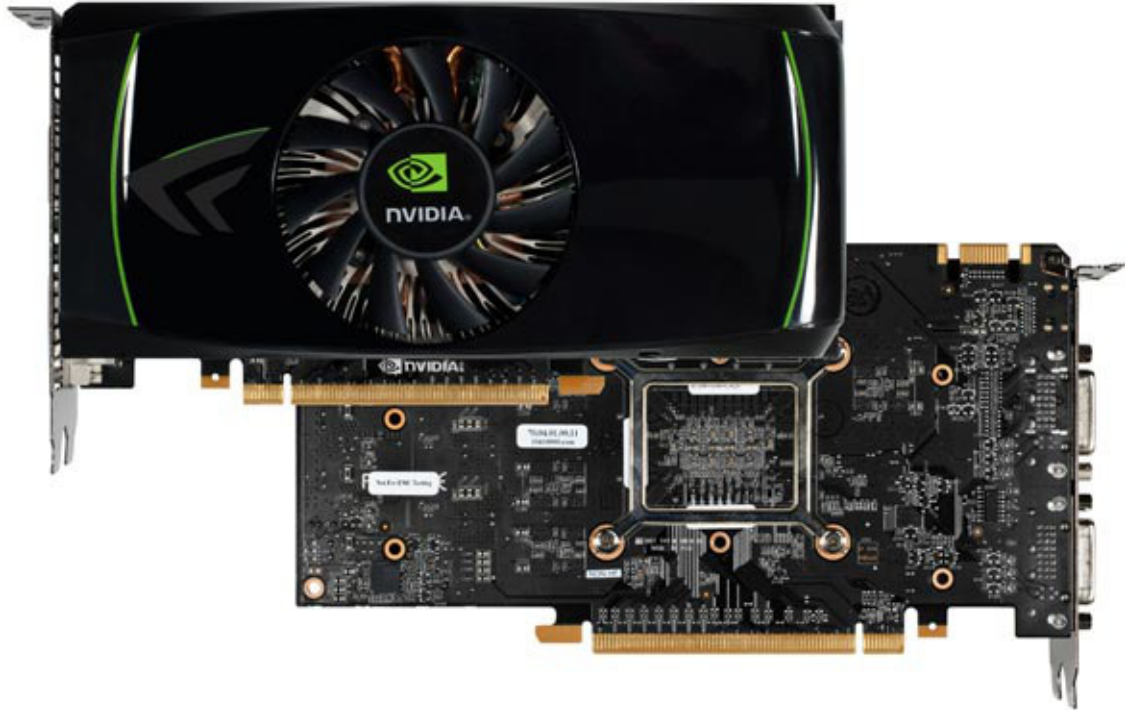
Figure 5.3: The NVIDIA GeForce GTX 460 GPU (NVIDIA is a Registered Trademark of NVIDIA Corporation).
