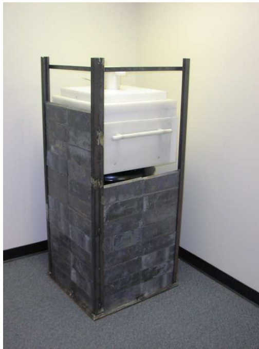
Figure 5.1. Assembled Neutron Howitzer with Lead Shielding
