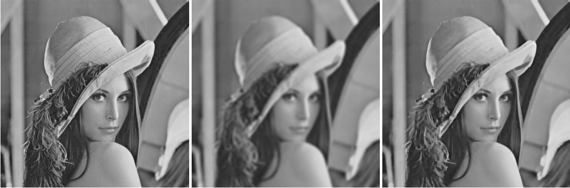
Figure 3.9: Image deblurring: original image(left), blurred and noisy image (middle), and deblurred image (right). The SNR of the blurred image is 11.01, and the SNR of the deblurred image is 17.23.
