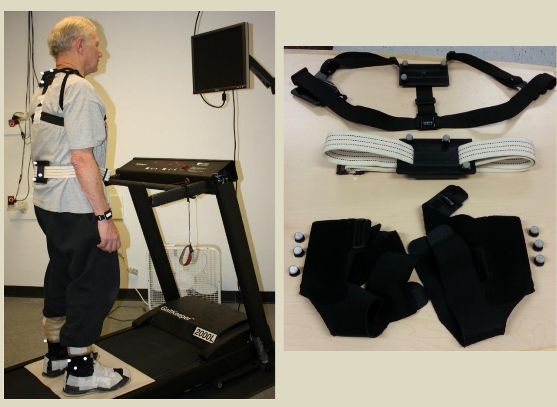
Figure 2.1. Left shows the marker setup worn by a subject (with sets of three reflective markers forming rigid bodies on the back, waist, and ankles) as well as the position of the monitor for presentation of feedback relative to the treadmill during experimental tasks. Right shows the individual components of the marker setup including a modified GoPro harness with rigid plate for back markers, gait belt with rigid plate for waist markers, and ankle braces for foot markers. Optitrack cameras tracked the rigid bodies' three-dimensional location and allowed for the calculation of step length, step time, and back angle.
