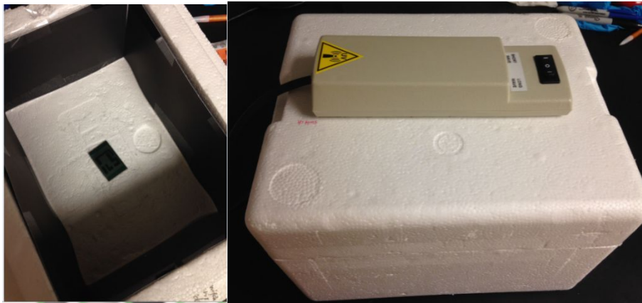
Fig 20. Configuration of UV Light Box. Surrounding walls are black to minimize UV scattering.
