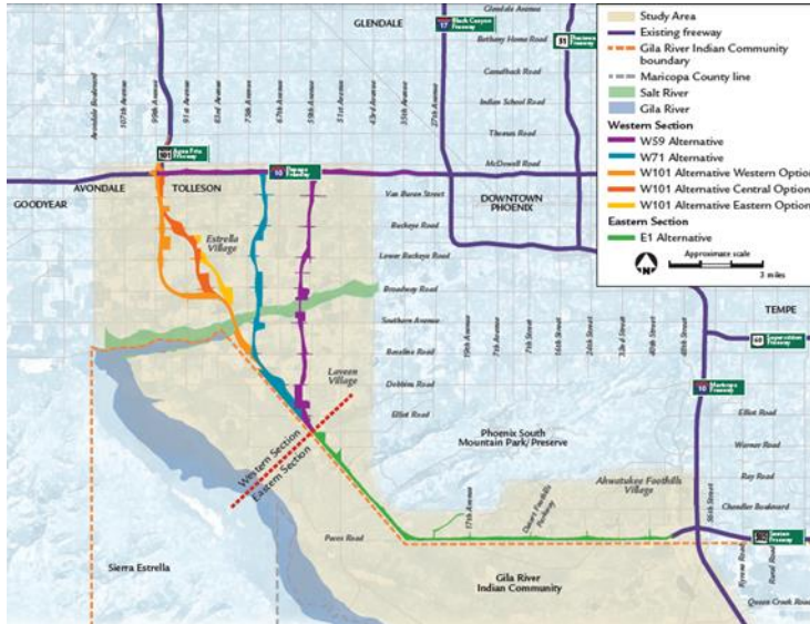
Figure 5.7. A map of the Loop 202 proposed routes depicts watersheds that would be affected by the freeway. The freeway would cross the Salt River, depositing toxins that would make their way into the Gila River. Source: South Mountain Freeway (Loop 202) DEIS and Section 4(f) Evaluation. P. 4-94.
