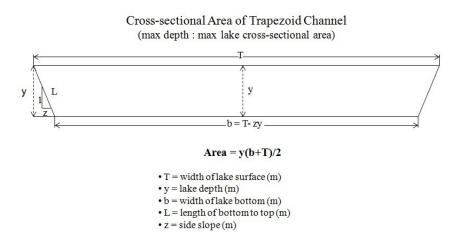
FIG.1. Trapezoid channel cross-sectional area used to calculate lake bathymetric profiles.
