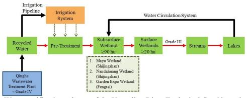
FIG.36. Water purification scheme of the Yongding River Ecological Corridor using subsurface and surface flow constructed wetlands.
