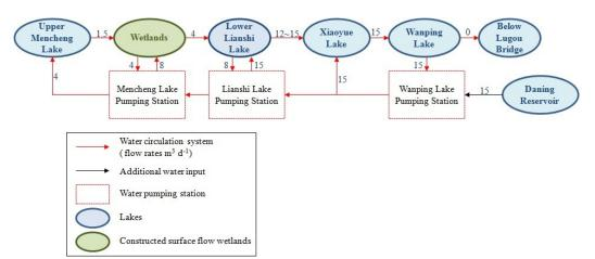
FIG.42. Water circulation system showing the hydrologic connections between lakes and constructed surface flow wetlands (listed are daily flow rates).
