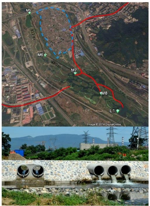
FIG. 49. Stormwater channels (outlined in red) feed into the Wetlands with water entering at M7. Outlined in dashed blue is a dense human settlement where wastewater has been seen going from the homes into the channels. The satellite image is of September 2013 taken from Google Earth, and the photo was taken at ground level at M7 in June 2013.
