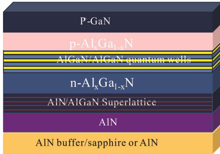
FIG. 6.1. Schematic diagram of DUV laser structure including p -barrier, MQWS active region, n -barrier, and AlN buffer layer on sapphire or AlN substrate.
