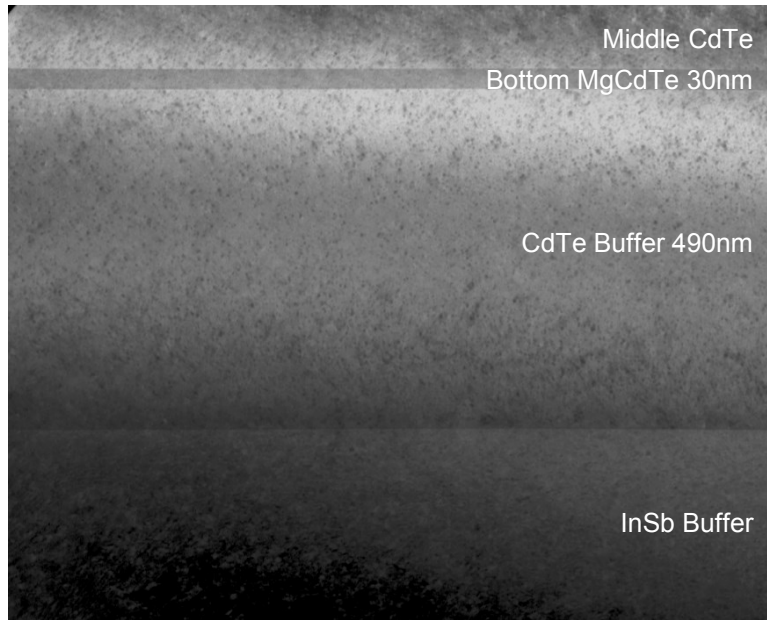
Figure 4.3. TEM image showing the lower portion of the CdTe/MgCdTe DH. *Image acquired by Jing Lu and Dr. David Smith at ASU.
