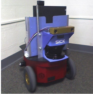
Figure 3.4: A Pioneer P3-AT on which the planner integration with OWQGs was verified.
