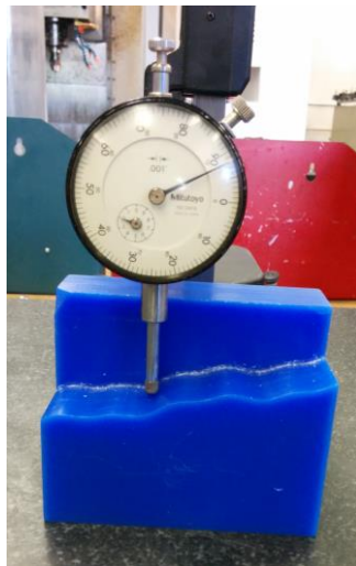
Figure 6.5: Manual Inspection of Part 6
