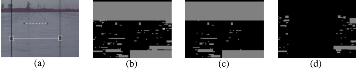
Figure 3.18: The Result of the At Least One Inside Constraint. (a) The Original Frame with White Solid Boxes Denoting a Tracking Pair and Black Lines Indicating the Bounds. (b) The Original Blob Set with a Blob in White Indicating the Specified Blob. (c) The Blobs That Can Be in a Pair with the Blob in White. (d) The Blobs That Cannot Be in a Pair with the Specified Blob.
