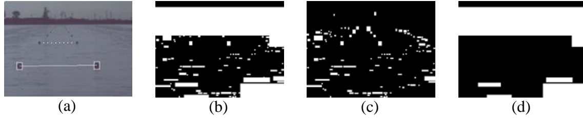
Figure 3.11: The Result of the Area Less Than Constraint. (a) The Original Frame with a White Solid Line Signifying a Tracking Virtual Buoys Pair and a White Dotted Line Indicating the Buoy Pair under Consideration. (b) Original Blobs. (c) Valid Blobs under the Constraint. (d) Invalid Blobs.
