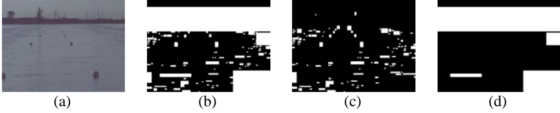
Figure 3.8: The Result of Applying the Unlocked Area Less Than Constraint. (a) Original Frame. (b) Original Blobs. (c) Valid Blobs under the Constraint. (d) Invalid Blobs.
