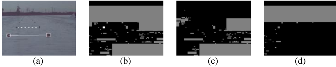
Figure 3.22: The Slope Greater Than Constraint. (a) The Original Frame. The White Solid Line Represents the Line Used to Determine the Threshold. The White Dotted Line Denotes the Pair under Consideration. (b) The Extracted Blob Set with the Specified Blob in White. (c) The Blobs Allowed to Be in a Pair with the Specified Blob by the Constraint. (d) The Blobs Rejected by the Constraint.
