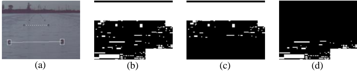
Figure 3.13: The Result of the Center Less Than Constraint. (a) The Original Frame with a Solid White Line Denoting a Tracking Buoy Pair and a Dotted Line Signifying the Pair under Consideration. (b) The Original Blob Set. (c) The blobs Valid under the Constraint. (d) The Invalid Blobs.
