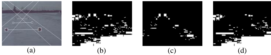
Figure 3.16: The Result of the In Lane Constraint. (a) The Original Frame. The Solid White Boxes Denote Tracking Buoys. The Diagonal Lines Illustrate the Lanes. (b) Original Blobs. (c) Blobs Validated under the Constraint. (d) Invalid Blobs.
