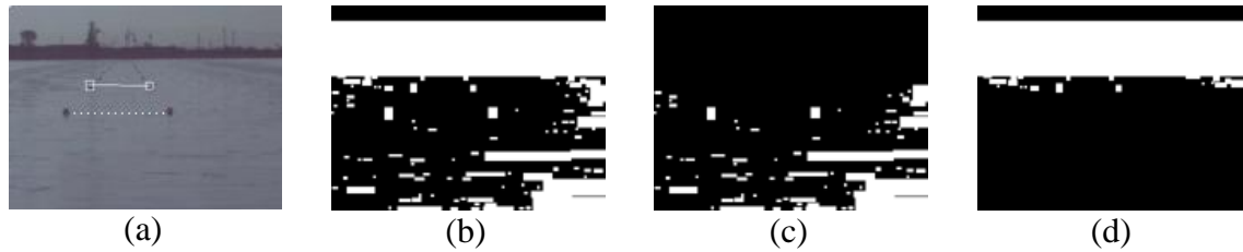
Figure 3.14: An Example of Firing the Center Greater Than Constraint. (a) The Original Frame with White Boxes Representing the next Furthest Pair of Tracked Buoys and a Dotted Line Denoting the Pair under Consideration. (b) Original Blobs. (c) The Valid Blobs under the Constraint. (d) Invalid Blobs.
