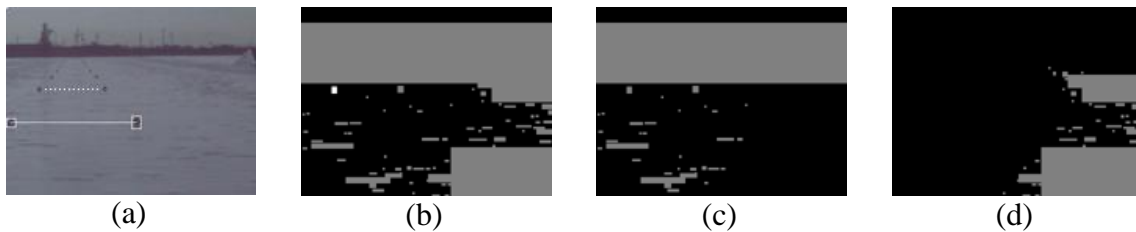
Figure 3.20: The Result of Applying the Distance Less Than Constraint. (a) The Original Frame with a White Solid Line Representing a Tracking Pair and a White Dotted Line Indicating the Pair under Consideration. (b) The Original Blob Set with the Blob All Pairs Are Built with in White. (c) The Blobs Allowed to Be in a Pair with the Specified Blob. (d) The Blobs That Cannot Be in a Pair with the Specified Blob.
