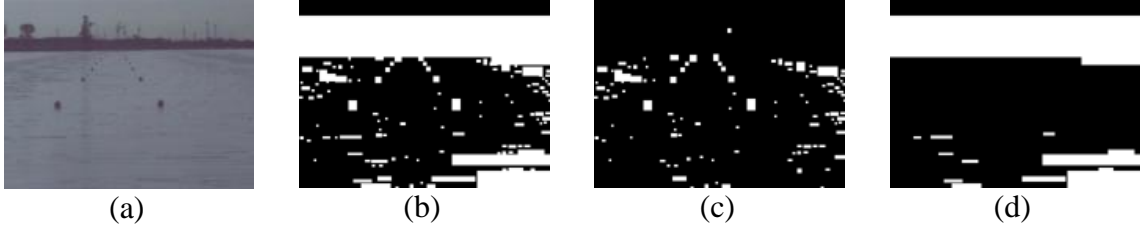
Figure 3.7: The Result of the Unlocked Dimensionality Constraint. (a) Original Frame. (b) Original Blob Set. (c) Valid Blobs under the Unlocked Dimensionality Constraint. (d) Invalid Blobs.
