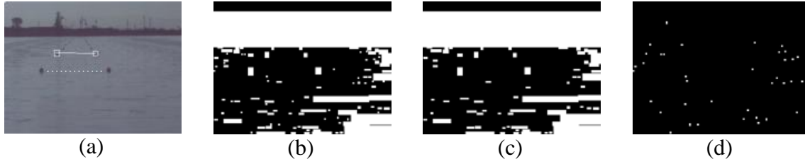
Figure 3.12: The Result of the Area Greater Than Constraint. (a) Original Frame. (b) Original Blobs. (c) Valid Blobs. (d) Invalid Blobs.
