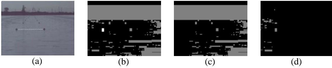
Figure 3.17: The Result of the Left Right Constraint. (a) Original Frame with a White Dotted Line between the Buoy Pair under Consideration. (b) The Original Blob Set with the Blob the System Considers the Left Blob in White. (c) The Blobs That Can Be in a Pair with the Specified Blob. (d) The blobs That Cannot Be in a Pair with the Specified Blob.
