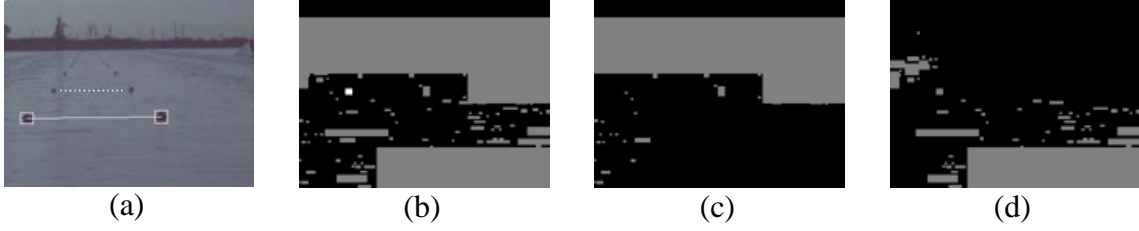
Figure 3.23: The Result of Applying the Pair Slope Greater Than Constraint. (a) The Original Frame with the Tracking Pair in White Boxes and a Solid White Line. (b) Original Blob Set with the Blob Tested in All Pairs in White. (c) The Blobs Allowed to Be in Pairs with the Specified Blob under the Constraint. (d) The Blobs Invalidated by the Constraint.
