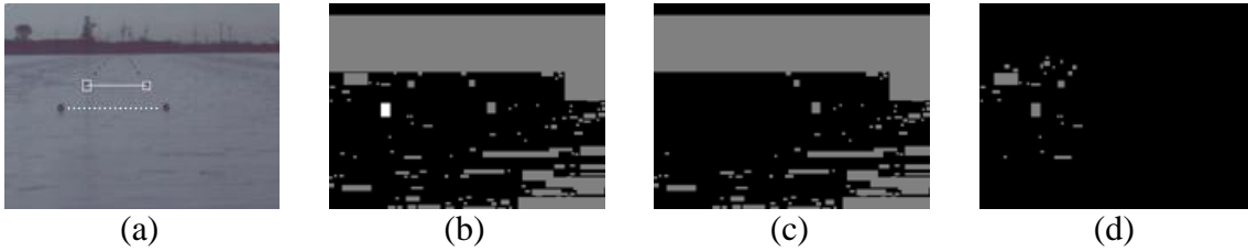
Figure 3.21: The Result of the Distance Greater Than Constraint. (a) The Original Frame with a White Dotted Box Denoting the Buoy Pair under Consideration and White Solid Boxes Representing a Tracking Pair. (b) The Original Blob Set with the Blob Tested in All Pairs in White. (c) The Blobs That Can Be in a Pair with the Specified Blob. (d) The Blobs That Cannot Be in a Pair with the Specified Blob.
