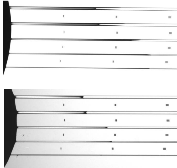
Figure 12. Image of PDMS Flow in Silicon Micro Channels with a Depth of 10 \mu\text{m} (top) and PTFE Coated Micro Channels with a Depth of 10 \mu\text{m} (bottom).
