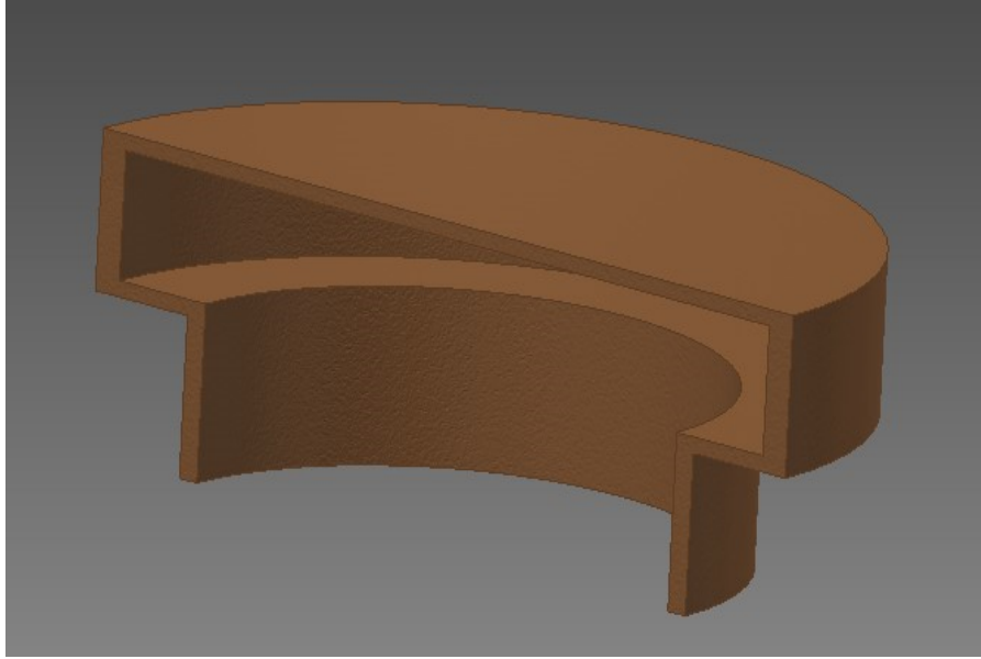
Figure 33. SSF with Cylindrical Inner Chamber (Vendrell, 2013)
