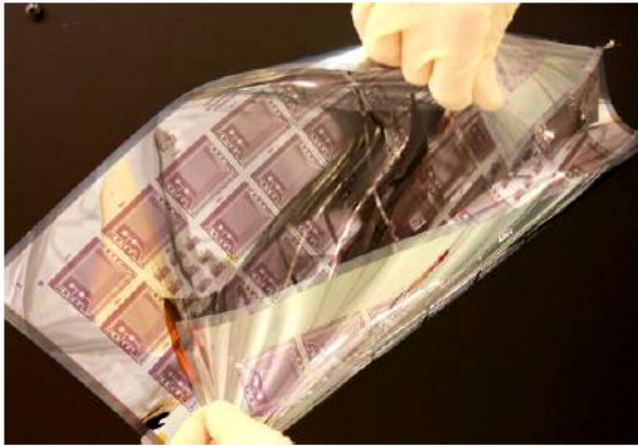
Figure 7. Flexible displays manufactured on a 370 mm x 470 mm gen2 PEN plastic substrate, after debond and prior to singulation. Bendable, but not stretchable.
