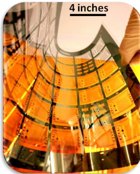
Flexible Display on 370 x 470mm Plastic (PEN) Substrate (photo courtesy ASU)
