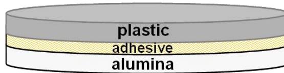
Adhesive Bond Flexible PEN Plastic Substrate to Alumina
