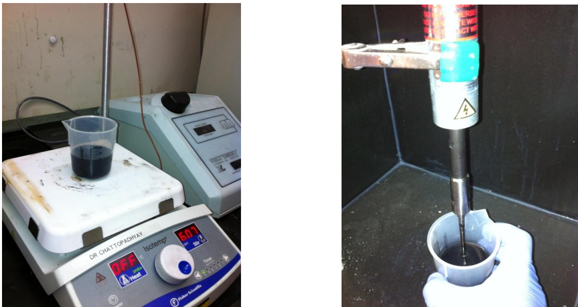
Figure 117. Mixture stirring and mixture sonication
