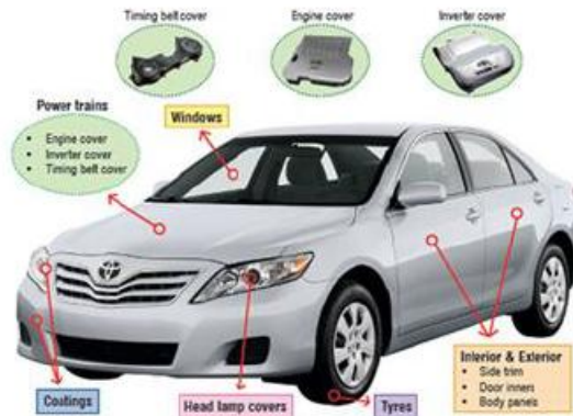
Figure 7. Illustration of the usage of polymer nanocomposites parts (nanowerk. 2014)
