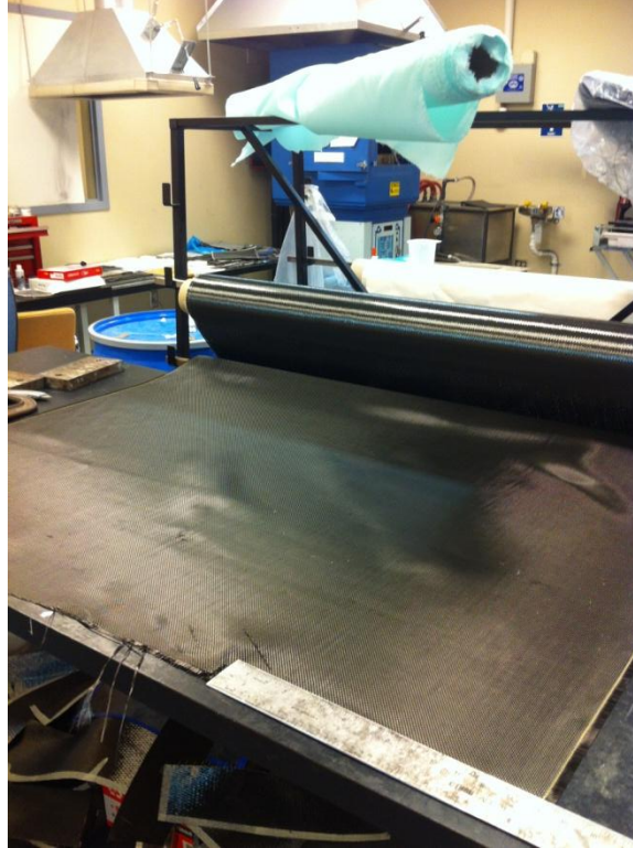
Figure 119. Plain weave carbon fiber fabrics used in manufacturing the specimens
