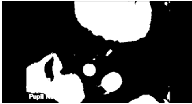
Figure 11: Resulting Binary Image at the Image Segmentation Step with Segmentation Performed Using a Fixed Global Threshold for all Pixels in the Image.
