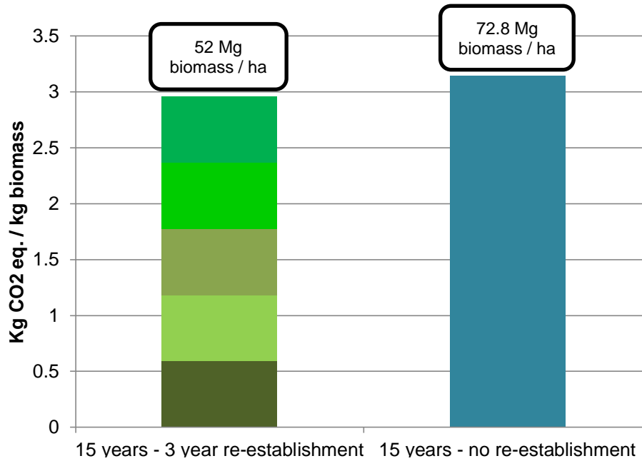
Figure 7 - Total GHG Emission Comparison of Re-establishing vs. Continuous Growth. The first bar represents the decision to re-establish the switchgrass every 3 years. The second bar represents allowing the switchgrass field to produce switchgrass for 15 years before re-establishment. Both bars include a year of preparation with no harvest. The textbox above gives the total biomass harvest during the 15 year time period.
