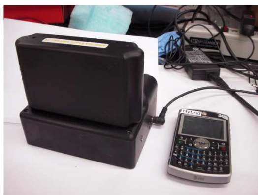
Figure 3-10. Operation of the two devices. (a) Wearable device measuring 1 ppm BTEX; (b) The docking station analyzing the pre-concentrated 1 ppm BTEX.
