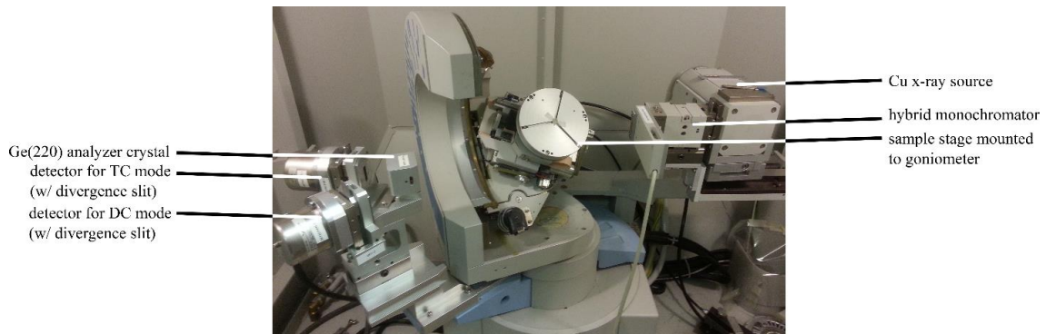
Fig. 15. PANalytical X'Pert Pro MR Diffractometer, Optical Scheme. LeRoy Eyring Center for Solid State Science.
