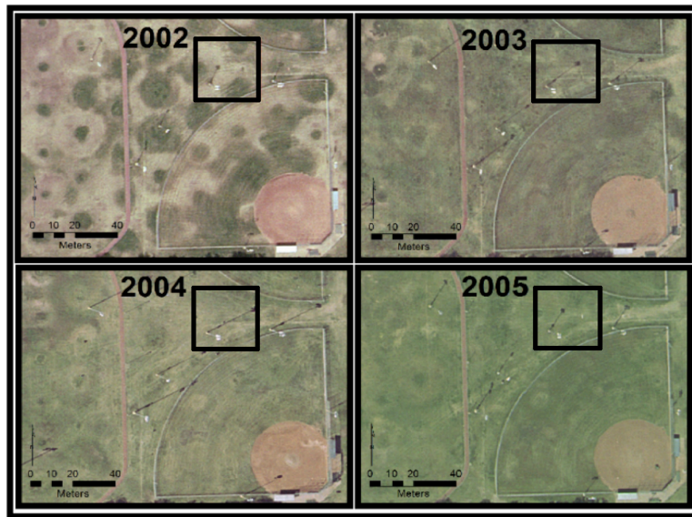
Figure 3-3. A Landsat pixel overlaid on the Assessor’s Office photography in 2002, 2003, 2004, and 2005. Based on the aerial photography, the health of the vegetation varies through these years, and so the intensity of the vegetation signal picked up by the Landsat sensors is expected to vary across the different years. This difference between area and intensity of vegetation may be one source of errors between the hand and mtmf datasets.
